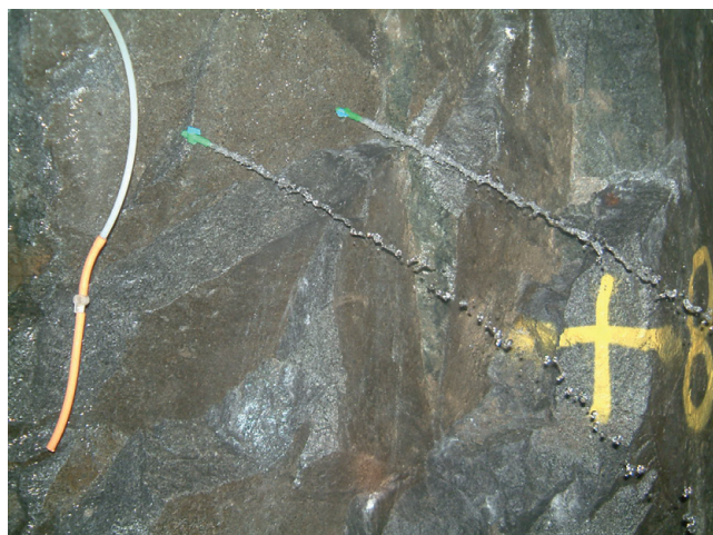
Fig. 6. Cluster of three mini-piezometers at chainage 860m in the Bhuiridh (eastern) aqueduct tunnel at the Cruachan Pumped Storage Hydro-power Station, drilled into granite and fitted with gas-tight taps (two of which were opened when the photograph was taken). The piezometers intersect a fracture some 0.2–0.3m behind the tunnel wall, which yields groundwater that has not yet encountered the air in the tunnel.
